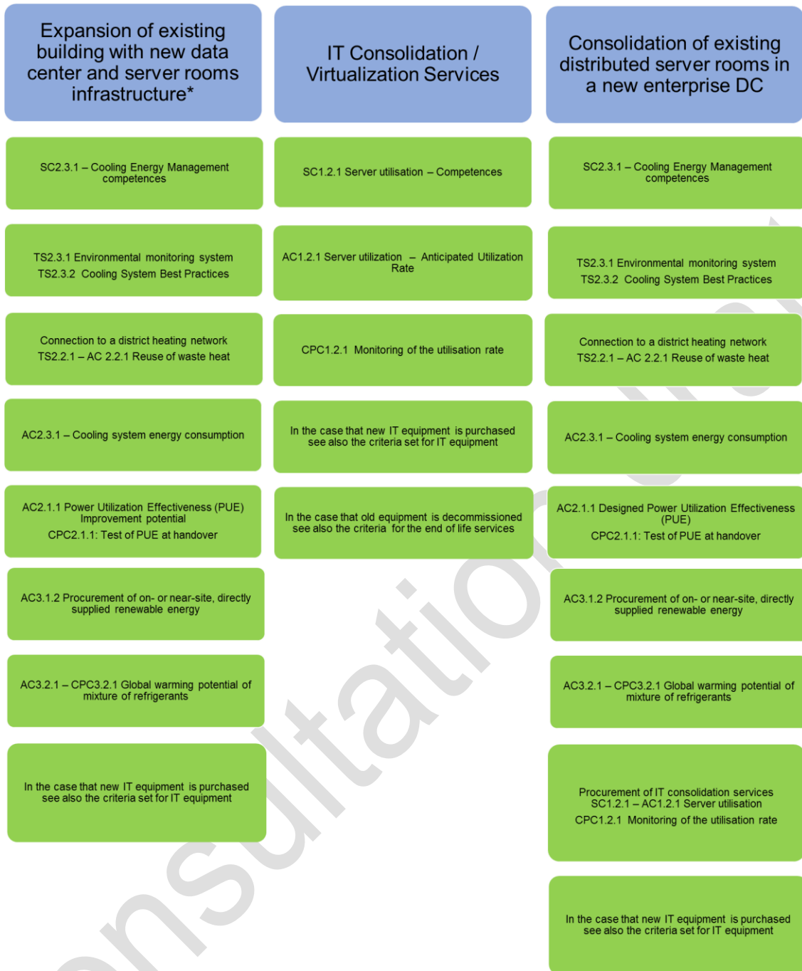
Figure 2: Applicability of GPP Criteria to retrofitting, expansion, consolidation and virtualization services (*this includes retrofitting such as upgrading electrical equipment or cooling system optimization)
